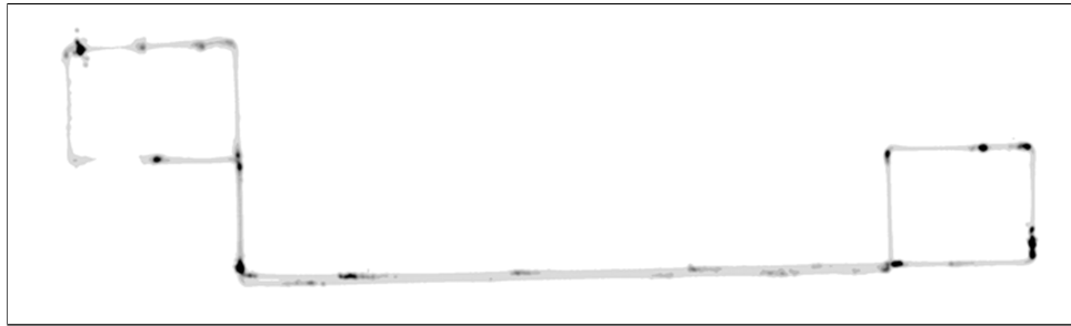
(b) Kernel density estimate of raw GPS points. Vehicles spend more time in the darker areas.
